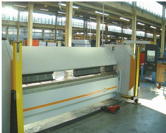
Depending on the application, folding machines can co-exist with press brakes, or can even replace them. They are ideal for short-run, Just-In-Time (JIT), or cellular-type bending applications.
